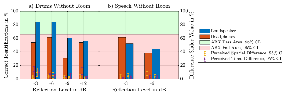
Fig. 5: Loudspeaker- and headphone-based listening test results for comparison between a reflection with an elevation angle of 10^\circ and 0^\circ at an azimuth angle of 0^\circ with varying reflection levels and source stimuli without added room
