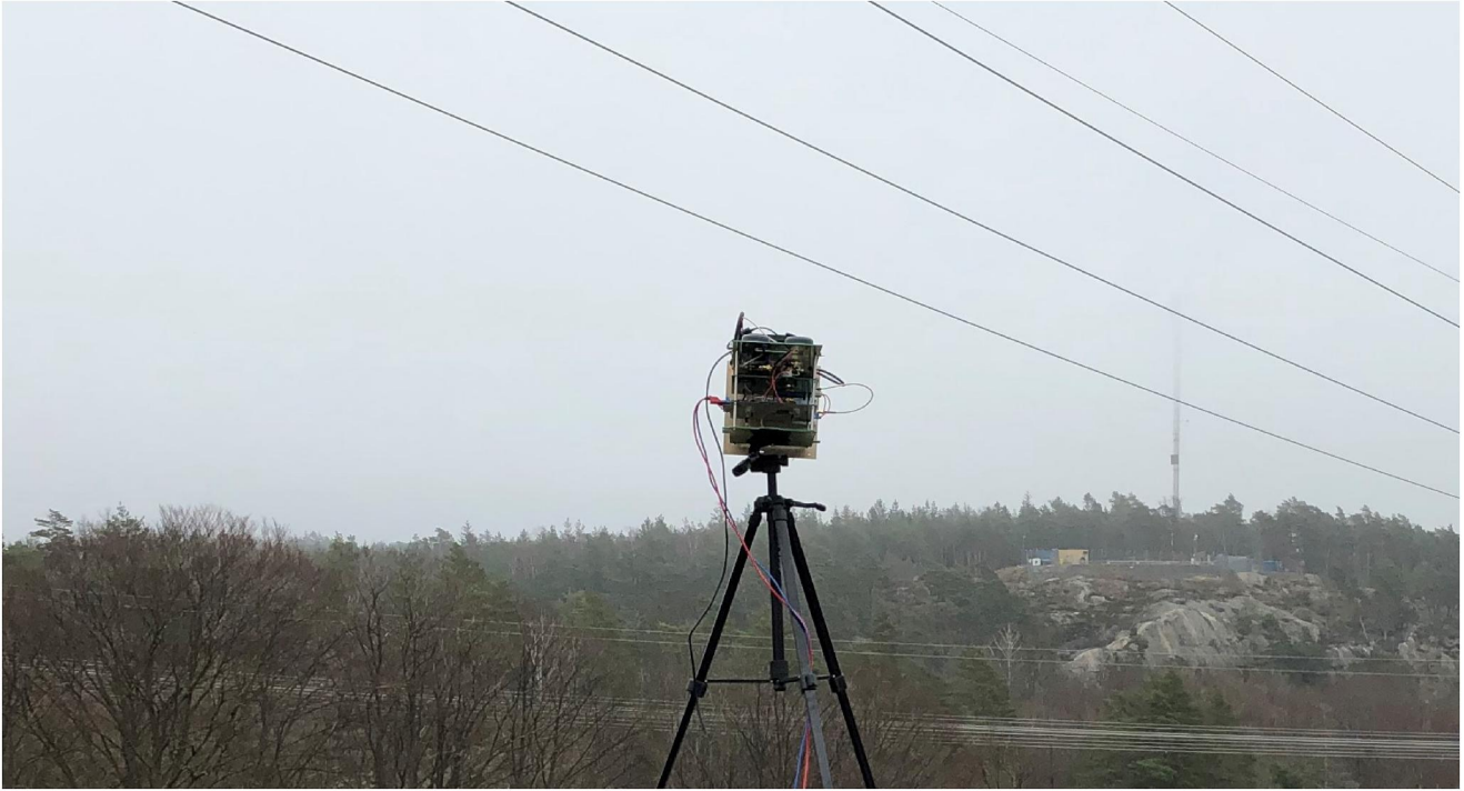
FIGURE A1 Location of the transmitter in the bistatic setting. The illuminated environment consists of several clutter objects, such as: trees, power lines, hills, radio towers, etc., which makes it a realistic setting for ground based radar systems
