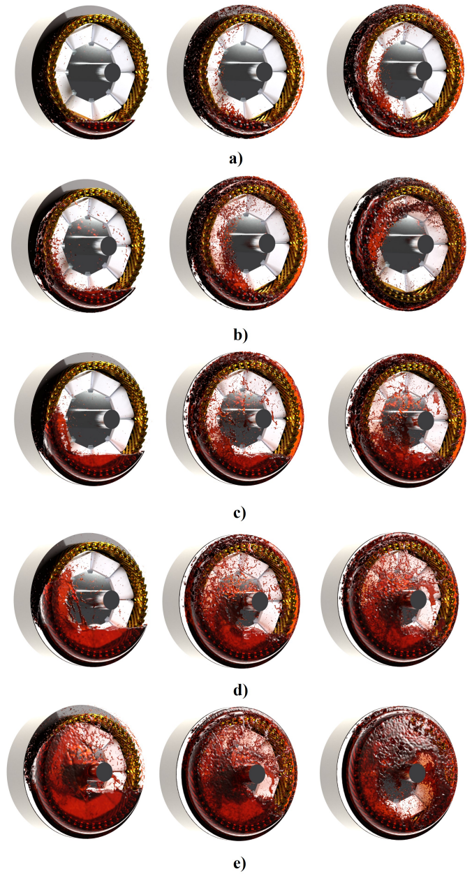
Fig. 7. Oil Splashing inside the motor at three rotor speeds 1000 rpm, 5000 rpm and 10000 rpm (from left to right) and different oil levels: a) 0.200 L; b) 0.300 L; c) 0.500 L; d) 0.700 L; e) 1.00 L.
