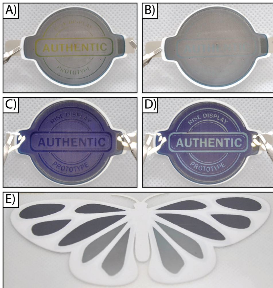
Figure 7. All-printed electrochromic displays in various designs highlight the potential of these multicolored materials. PEDOT/PPy blends in an authentic label design showing the A) reduced and B) oxidized states. PEDOT/PProDOT-Me 2 blends in an authentic label design showing the C) reduced and D) oxidized states, and E) a butterfly design using the PEDOT/PProDOT-Me 2 blend with the top half section being reduced and the lower half being oxidized.
