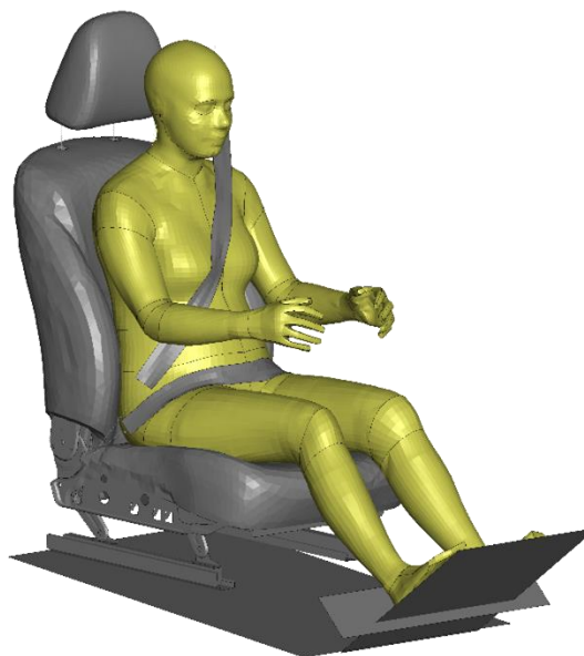
Figure. 3.11 The VIVA+ female occupant model at the time 0 ms before the crash pulses were applied.
