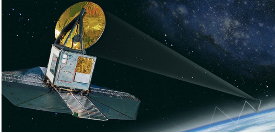
Figure 5.2: Upward and downward scanning of the atmosphere by Odin/SMR.
