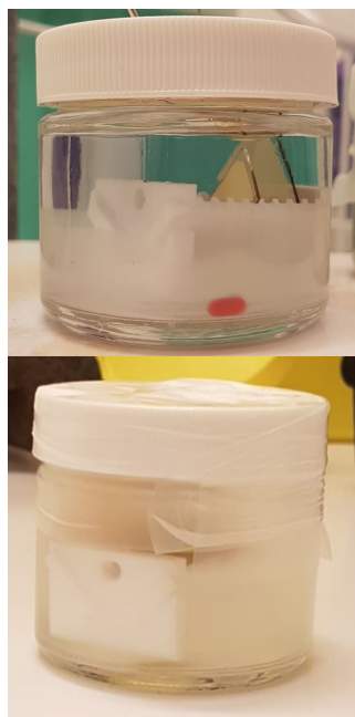
Figure 5.6: Turbid PNIPAM polymerizations solutions during ARGET-ATRP. MeOH volume fractions are between 0.25 and 0.5 in this case.
