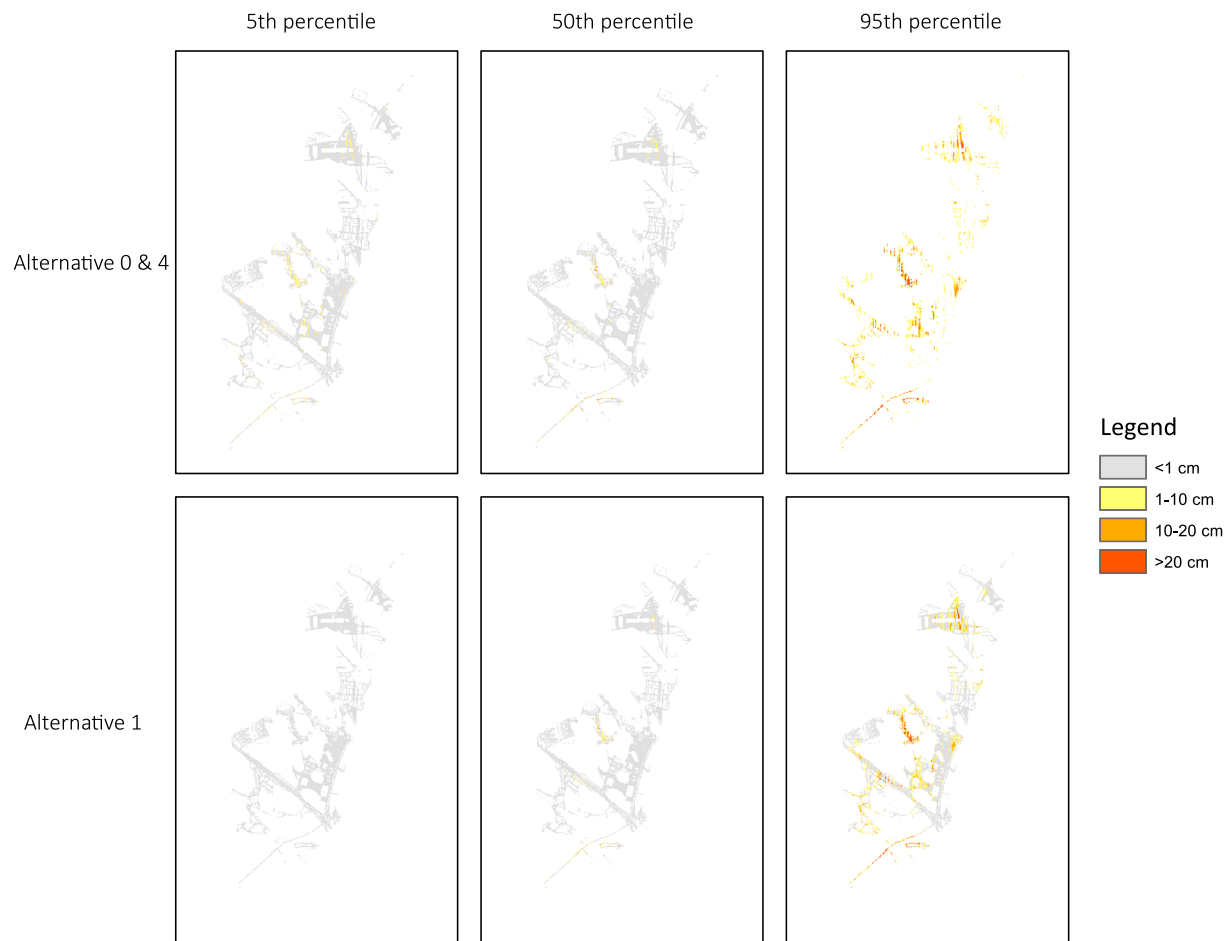
Fig. 5. Result from the subsidence simulations for the 5th, 50th and 95th percentile. The upper row shows the result for risk mitigation alternative 0 and 4 and the lower row shows the result for risk mitigation alternative 1. Alternative 2 and 3 is not included in the Fig. since they both includes artificial recharge that counteracts any groundwater lowering which eliminates the risk of subsidence.
