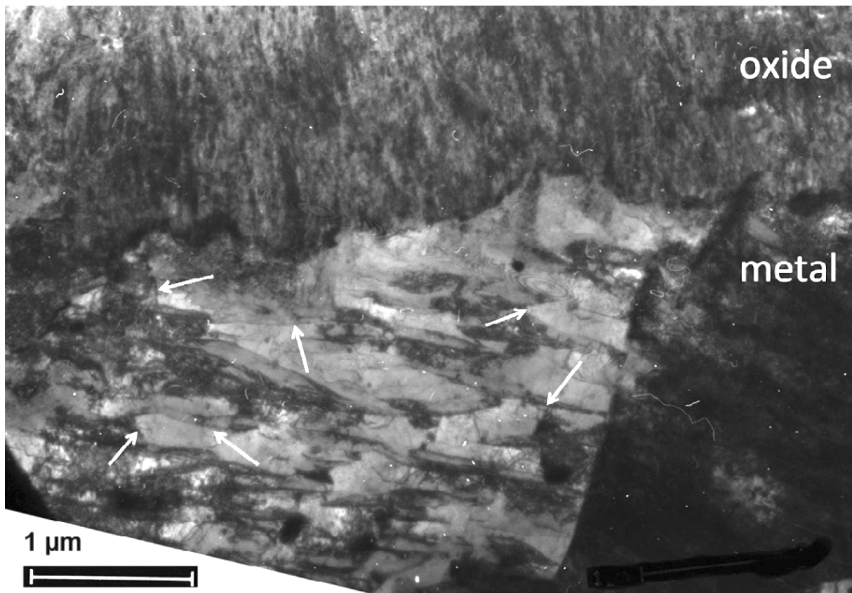
Figure 5.2: TEM micrograph of the metal/oxide interface in autoclave-corroded Zircaloy-2. Arrows indicate subgrain boundaries in the metal. Republished with permission from Elsevier, [100].
