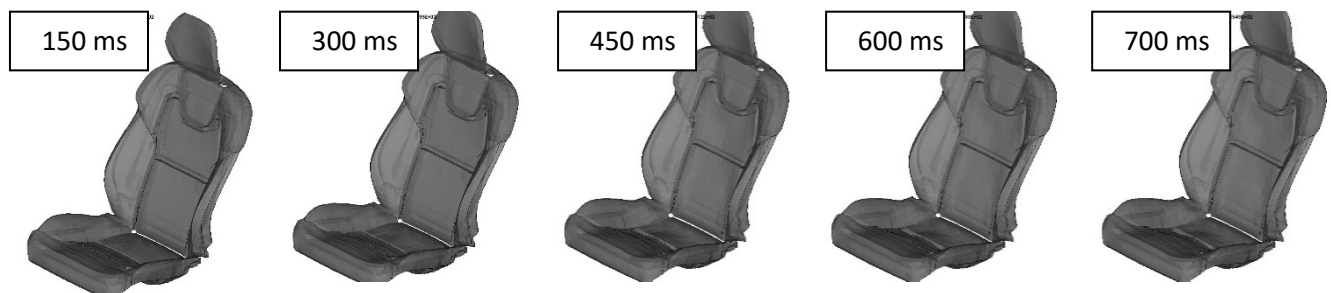
Fig.B.4. HBM positioning, seat squashing. The contact between the occupant and the seat deforms the seat foam. In the 300–450 ms time interval, the occupant is pulled into position. Between 450 ms and 700 ms, the external force is stopped and the HBM is allowed to reach equilibrium with the seat under gravity loading.
