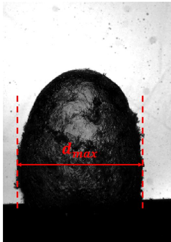
Figure 3. The ‘pear-like’ shape of the airgun bubble in a free field.
