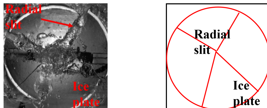
Figure 9. Radial slits pattern when H = 0.53 , T = 0.27 .
