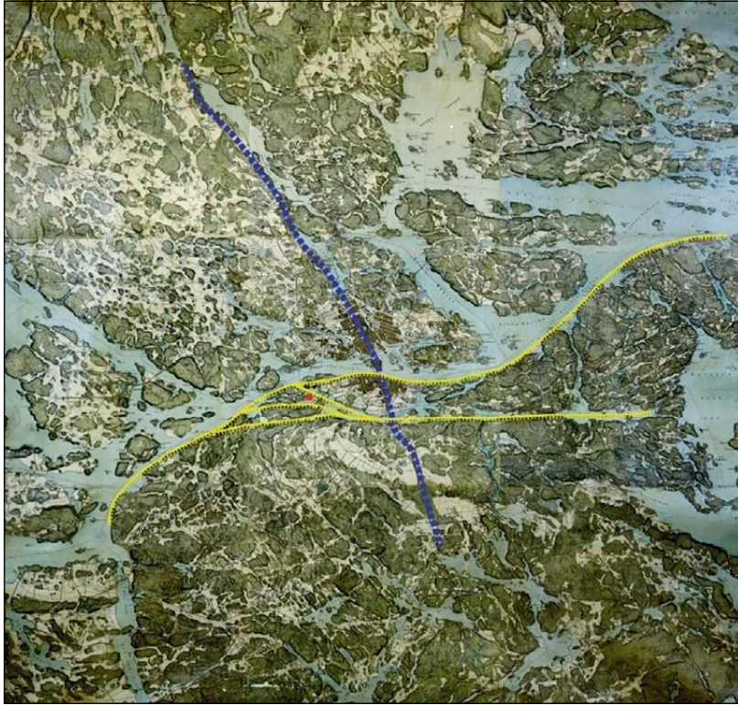
Figure 3: On the map, parts of the geological main structure are marked: fault slopes (yellow), the ridge Stockholmsåsen (blue). Lövholmen is marked by the red dot. A military map from 1861 is used as underlay for the sketch. Source: Historical maps, the City museum of Stockholm (SSA)
