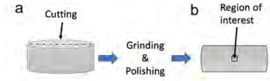
Figure 4.4: (a) Deformed sample with the cutting plane illustrated. (b) The revealed cross-section of a cut, ground and polished sample with the region of interest marked with the rectangle.
