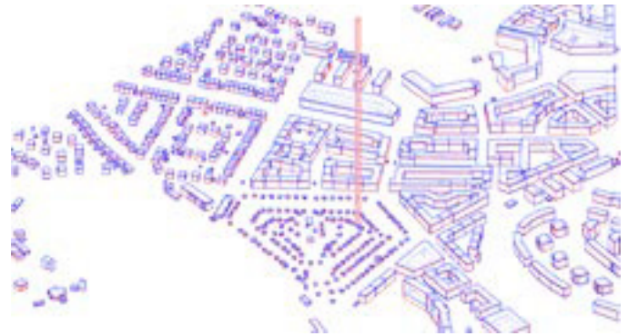
Fig. 5. Mesh comparison between results of FME and DTCC Builder workflows (Red - FME, Blue - DTCC Builder)
