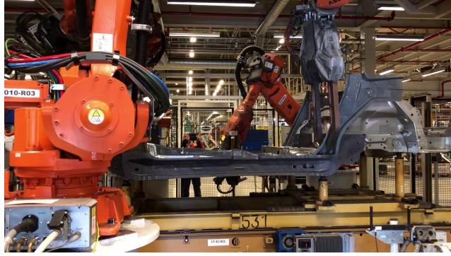
Figure 2.1: A welding station from Volvo Cars.
