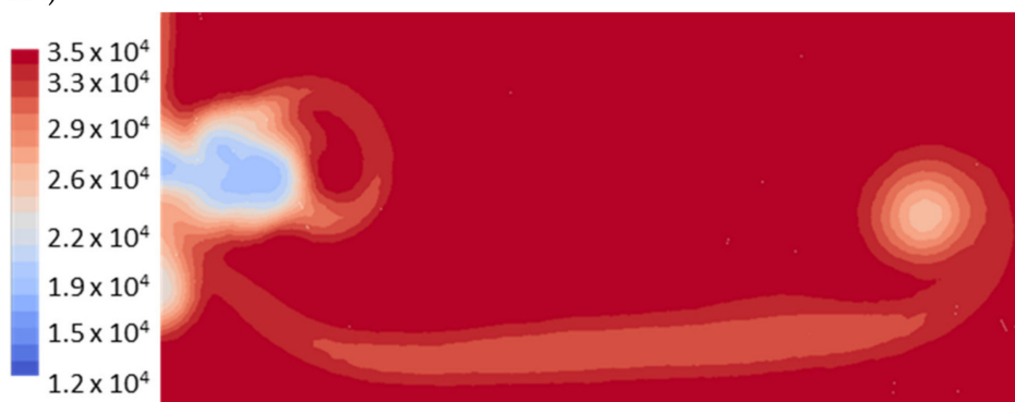
Figure 20. Pathlines towards the inlet of the engine (top left), the contour of the Mach number in the plane of fan inlet (top right), and the contours of the total pressure [Pa] in the planes of interest (From the second to the last: Plane 1, Plane 2 and Plane 3), results from the 3D simulation of short fuselage.
