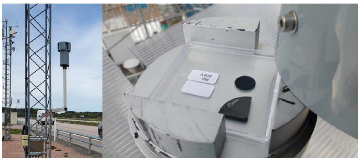
Figure 12. Sigma 2 sampler at Testsite E18. Photo: Mats Gustafsson, VTI and David Jaramillo, Particle Vision.
