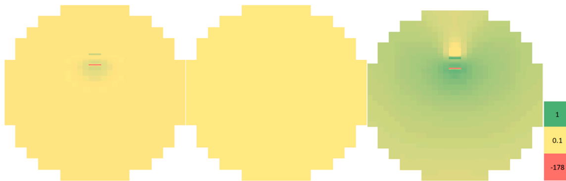
Fig. 28. The phase of thermal neutron noise in the maximized leakage core loading (at the mid-height position of the detector installation) - Left: Total noise, Center: Point kinetics component, Right: Shape function.
