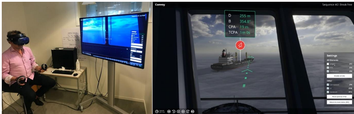
Figure 6 (Left) An exocentric perspective in VR/AR test set-up showing how the researcher can monitor both the users' behavior and have the same visuals as the user in VR on the TV screen. (Right) A screen capture of the egocentric perspective of what the user sees in the VRROS during the convoy scenario.
