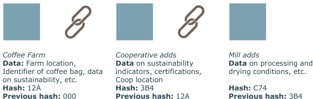
Fig. 1. The basic principles of a blockchain for a hypothetical coffee supply chain.
