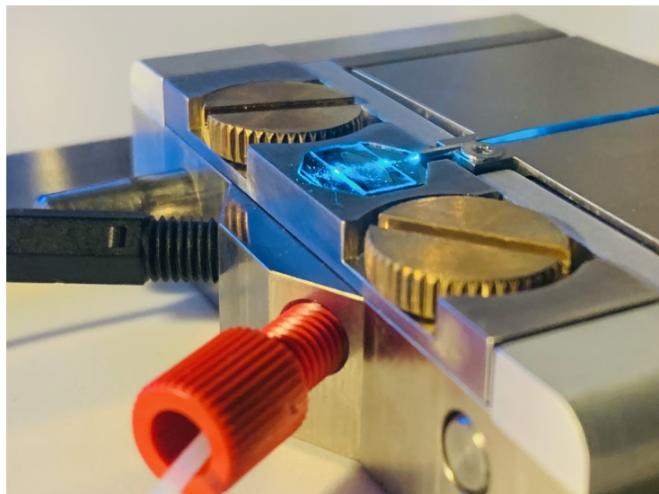
Figure 4.4: Picture of a waveguide chip with an integrated flow cell as implemented in paper IV, placed in the Nanolyze TM Vision fluid handling and laser coupling system.
