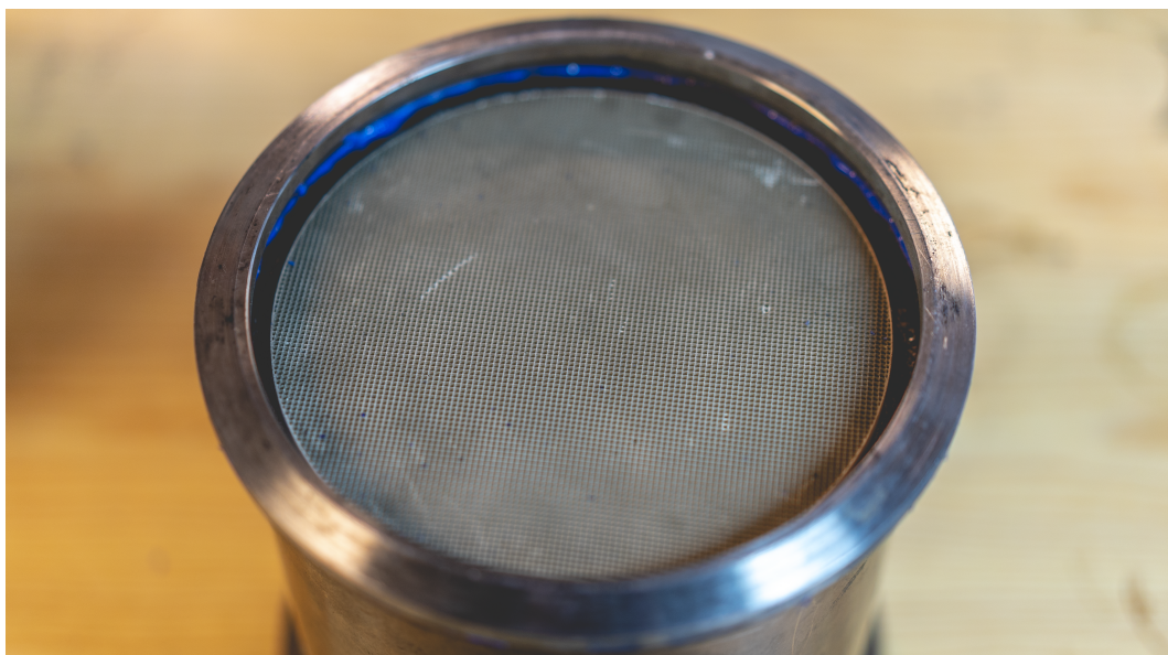
Figure 2.2: Photograph of a 400 CPSI ceramic monolith placed inside a metal casing.
