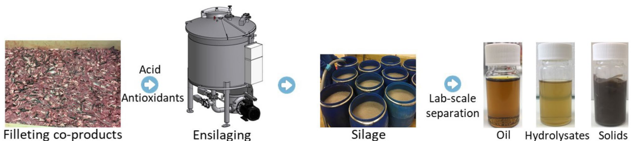
Fig. 1 Pilot-scale ensilaging of herring filleting co-products and subsequent lab-scale separation of silage into fish oil, protein hydrolysates, and solids. The silage was separated into oil, protein hydrolysates, and solids by centrifugation of the silage at 3000–8500 × g for 2–20 min
