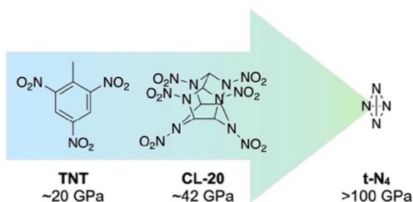
Figure 1. Detonation of energetic materials is one way to explore the effect of high pressure on chemistry. Shown are trinitrotoluene (TNT), Hexanitrohexaazaisowurtzitane (CL-20) and tetrahedral nitrogen (t-N 4 ).
