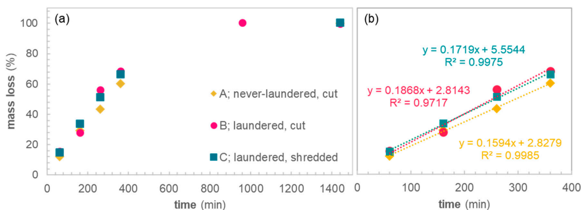
Figure 2. (a) Mass loss of samples A, B, and C, with increasing accessibility during hydrolysis, (b) linear fits to the first 4 datapoints of each sample shown in (a).
