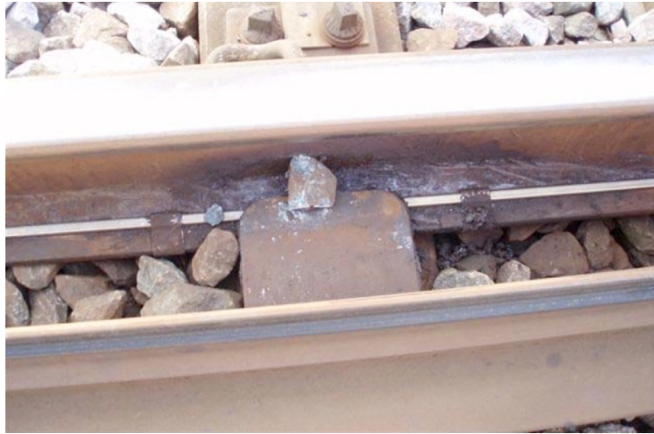
Figure 6 The ballast stone that caused the derailment in Hamra 2010. From accident report 2010. Picture courtesy Trafikverket.
