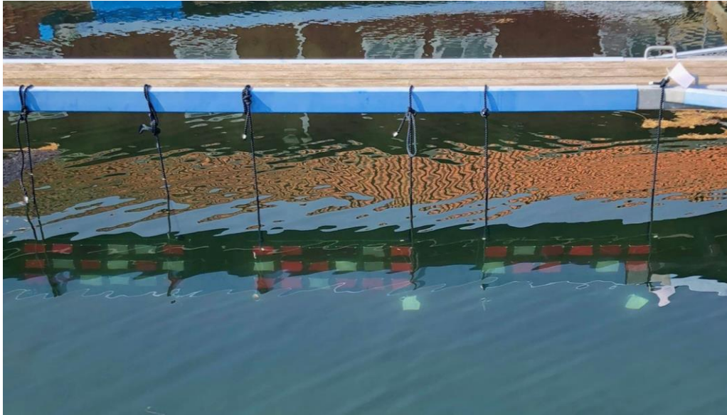
Figure 17. Arrangement of static panels in the field trials. Picture shows the experiment at Kristineberg marine research & innovation center (Atlantic region according to new ERA tool).
