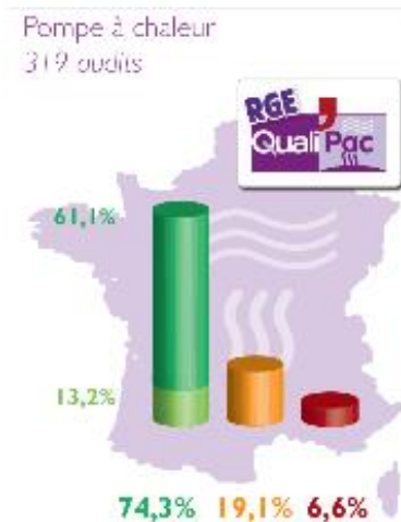
Figure 32 Results of the audits operated in the year 2012 by Qualit'EnR on 319 heat pump installations under the quality label QualiPAC. (dark green: excellent, light green: good, orange: insufficient, red: failing)
