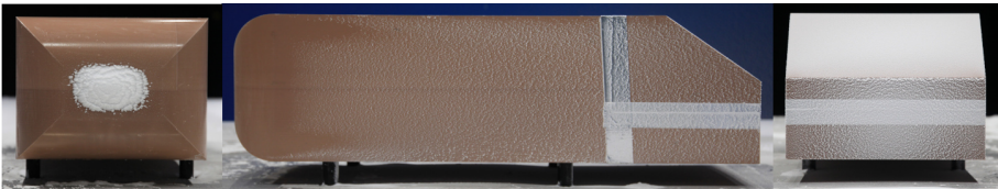
Figure C.5: Experimental trial on the Ahmed body at 20 km/h showing front, side, and rear surfaces.
