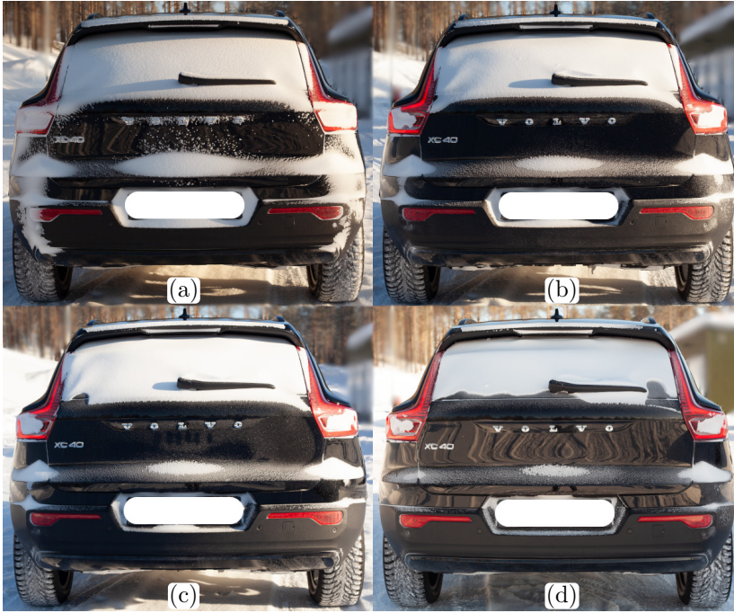
Figure A.1: Snow accumulation during resuspension test at rear view of Vehicle A at T = -12 \pm 3 \text{ }^\circ\text{C} : (a) 40 km/h for 12.5 km; (b) 40 km/h for 12.5 km and 70 km/h for 12.5 km; (c) 40 km/h for 12.5 km and 70 km/h for 25 km; (d) 40 km/h for 12.5 km, 70 km/h for 25 km and 70/90 km/h for 12.5 km.
