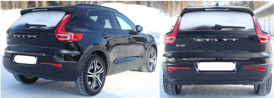
(b) Third-party contamination test of Vehicle A while driving at 70 km/h for 50 km at T = -8 \pm 2^\circ\text{C} .
