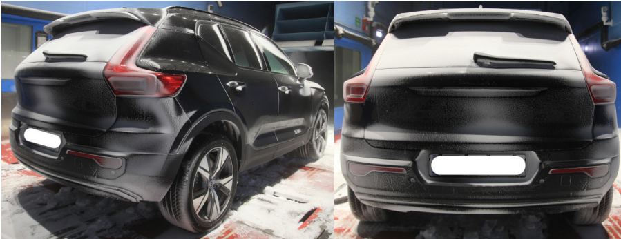
(a) Wind tunnel measurement of vehicle C for testing in 30 min with U_\infty = 70 km/h at T = -15^\circ\text{C} .
