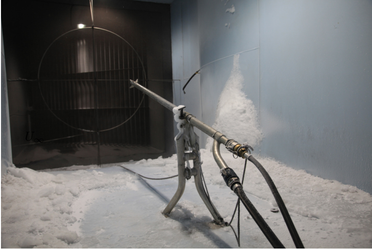
Figure 3.2: Snow cannon in wind tunnel where the cannon is placed in head-wind direction.
