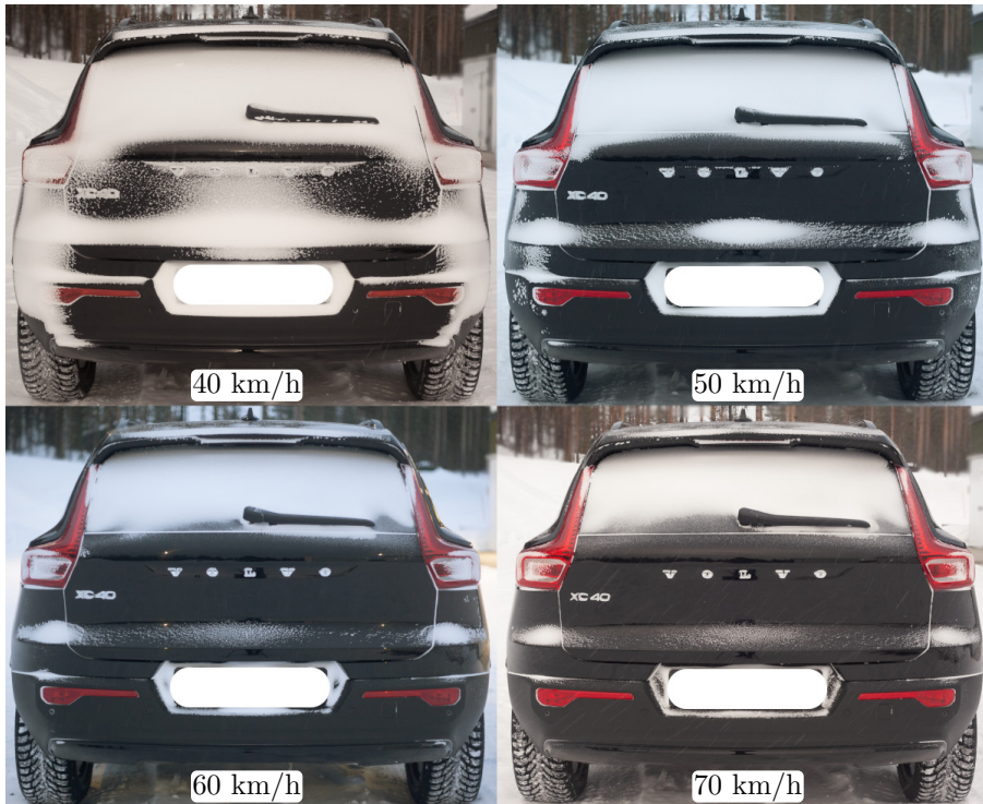
Figure 3.4: Snow accumulation at a rear view of Vehicle A after driving for 25 km at the speeds; 40, 50, 60, and 70 km/h at T = -8 \pm 2^\circ\text{C} .
