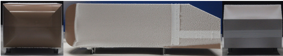
Figure C.2: Experimental trial on the Ahmed body at U_\infty = 115 km/h for \beta = 25^\circ showing front, side, and rear surfaces.
