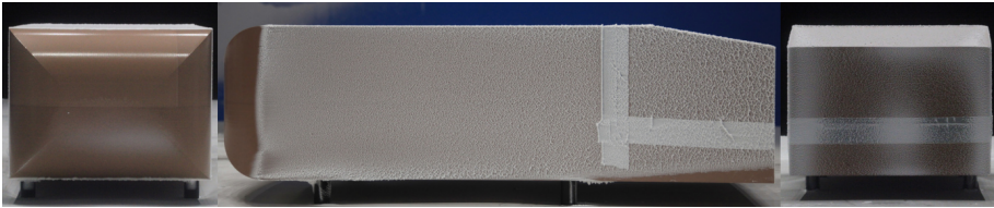
Figure C.1: Experimental trial on the Ahmed body at U_\infty = 115 km/h for \beta = 10^\circ showing front, side, and rear surfaces.
