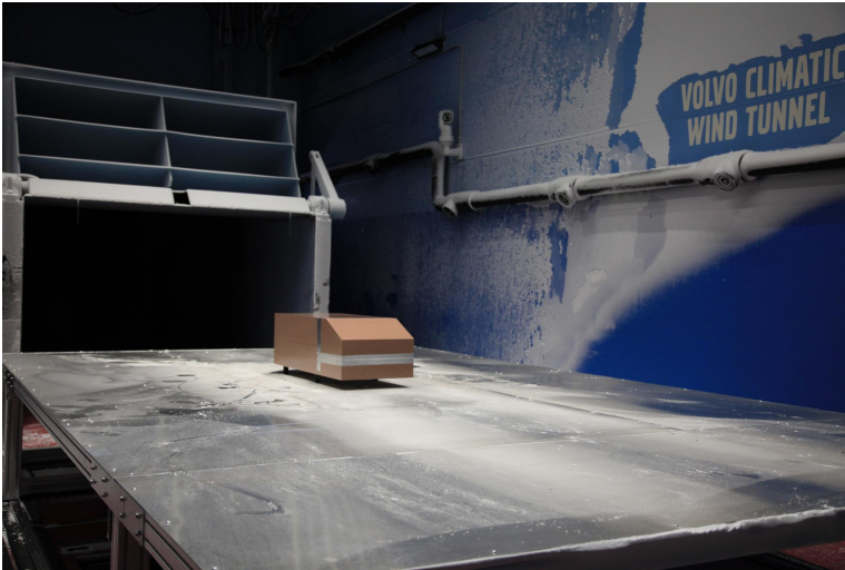
Figure 6.2: The Ahmed body with slant angle \beta = 35^\circ placed on the metal table in the wind tunnel.
