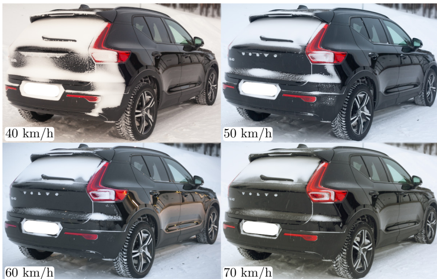
Figure 3.5: Snow accumulation at an isometric rear view of Vehicle A after driving for 25 km at the speeds; 40, 50, 60, and 70 km/h at T = -8 \pm 2^\circ\text{C} .
