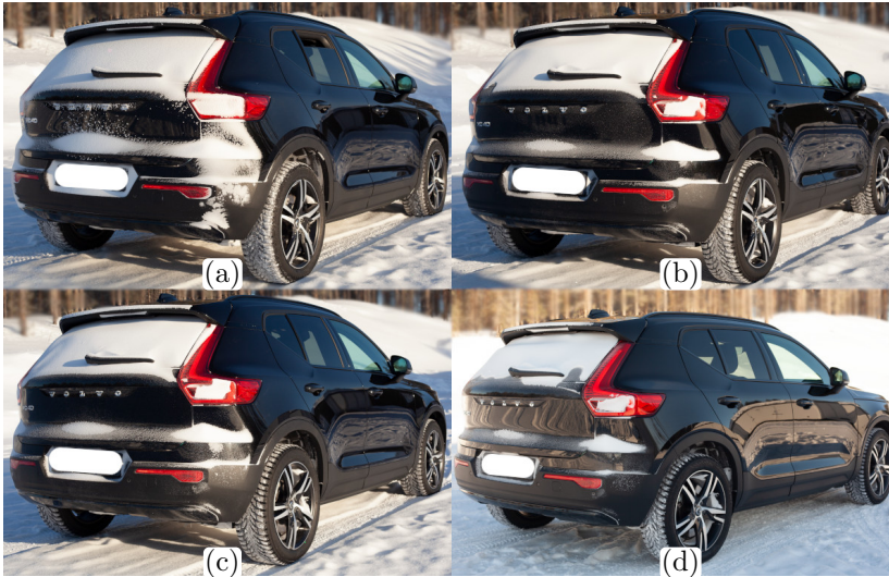
Figure A.2: Snow accumulation during resuspension test at isometric side rear view of Vehicle A at T = -12 \pm 3 \text{ }^\circ\text{C} : (a) 40 km/h for 12.5 km; (b) 40 km/h for 12.5 km and 70 km/h for 12.5 km; (c) 40 km/h for 12.5 km and 70 km/h for 25 km; (d) 40 km/h for 12.5 km, 70 km/h for 25 km and 70/90 km/h for 12.5 km.
