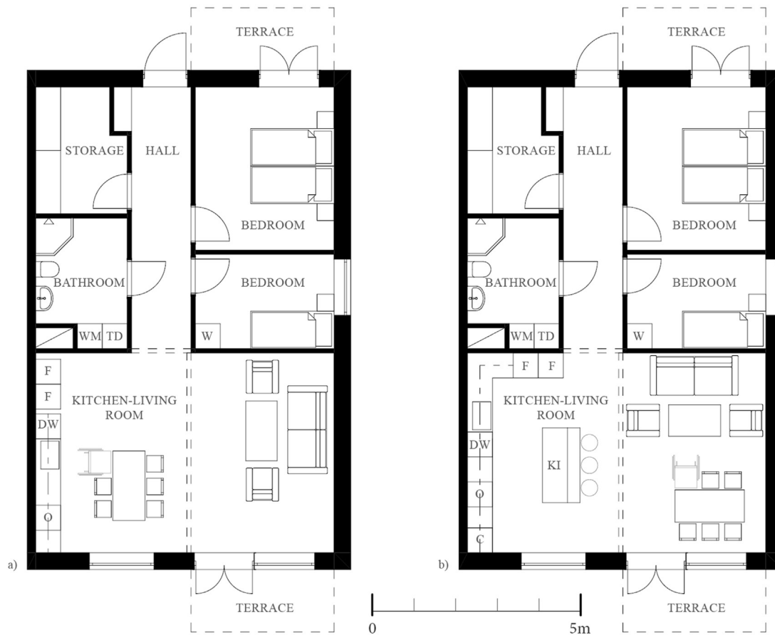
Fig. 10 Exemplifying the concept 'rearrange': (a) An apartment floorplan (74.1 m 2 ) with the planned kitchen (Source: illustration by Anita Ollár, original floorplan by Semrén & Månsson Arkitektkontor). (b) A possible rearrangement of the kitchen typology (proposal by Anita Ollár). C: cupboard, DW: dishwasher, F: fridge and freezer, KI: kitchen island, O: oven and stove, TD: tumble dryer, W: wardrobe, WM: washing machine.
