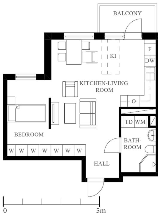
Fig. 20 Apartment floorplan (47.6 m 2 ) with free floor area for installing a kitchen island or reconfiguring the kitchen typology (Source: illustration by Anita Ollár, original floorplan by Tengbom). DW: dishwasher, F: fridge and freezer, KI: kitchen island, O: oven and stove, TD: tumble dryer, W: wardrobe, WM: washing machine.
