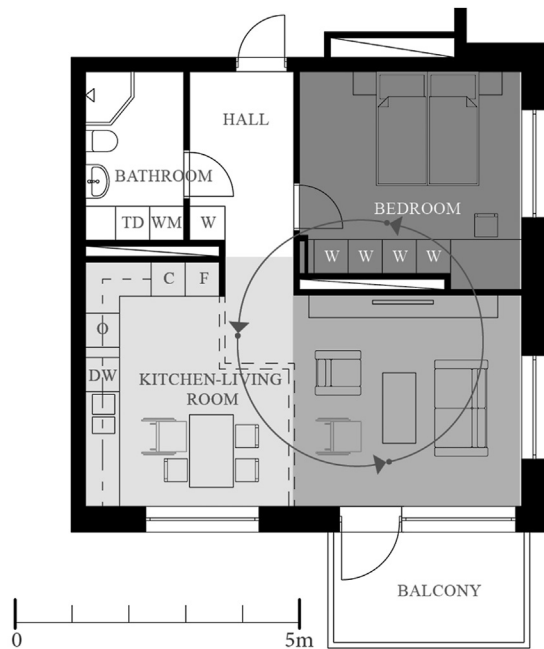
Fig. 17 Apartment floorplan (65 m 2 ) with multiple shafts accessible from several rooms with windows (Source: illustration by Anita Ollár, original floorplan by Tengbom). C: cupboard, DW: dishwasher, F: fridge and freezer, O: oven and stove, TD: tumble dryer, W: wardrobe, WM: washing machine.
