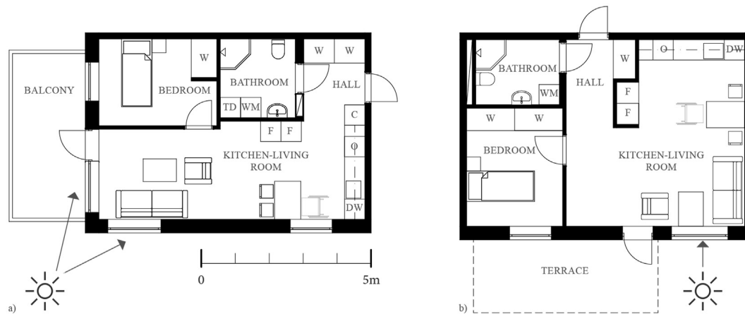
Fig. 7 Apartment examples with (a) two perpendicular and (b) one daylight directions (Source: illustration by Anita Ollár, original floorplans by Efem Arkitektkontor). C: cupboard, DW: dishwasher, F: fridge and freezer, O: oven and stove, TD: tumble dryer, W: wardrobe, WM: washing machine.
