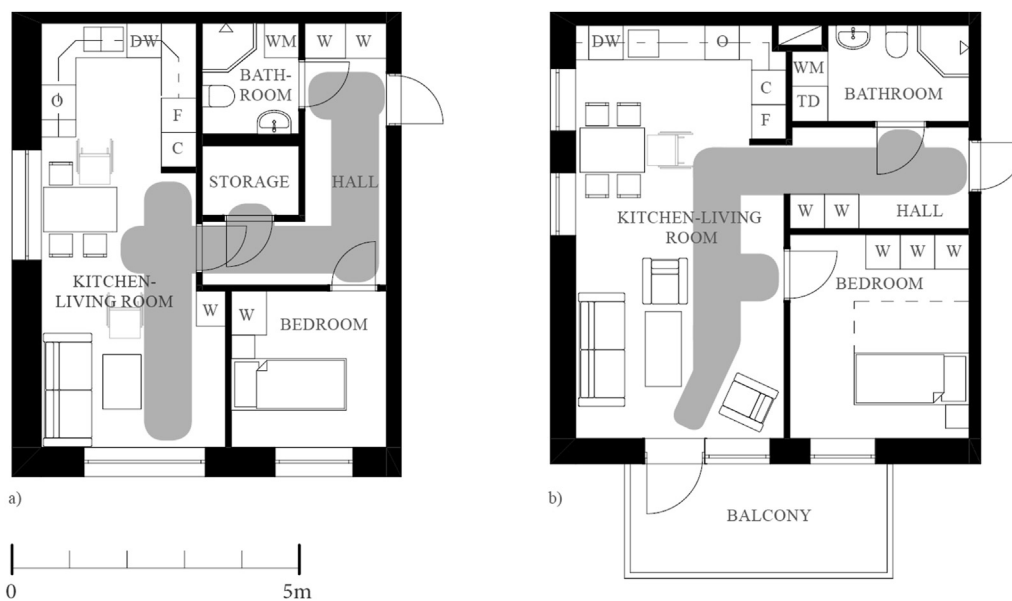
Fig. 16 Apartment floorplan with (a) increased number of doors and traffic zones (46.9 m 2 ; Source: illustration by Anita Ollár, original floorplan by White Arkitekter) and with (b) fewer doors and traffic zones, allowing extra free floor area (49.7 m 2 ; Source: illustration by Anita Ollár, original floorplan by Tengbom). C: cupboard, DW: dishwasher, F: fridge and freezer, O: oven and stove, TD: tumble dryer, W: wardrobe, WM: washing machine.
