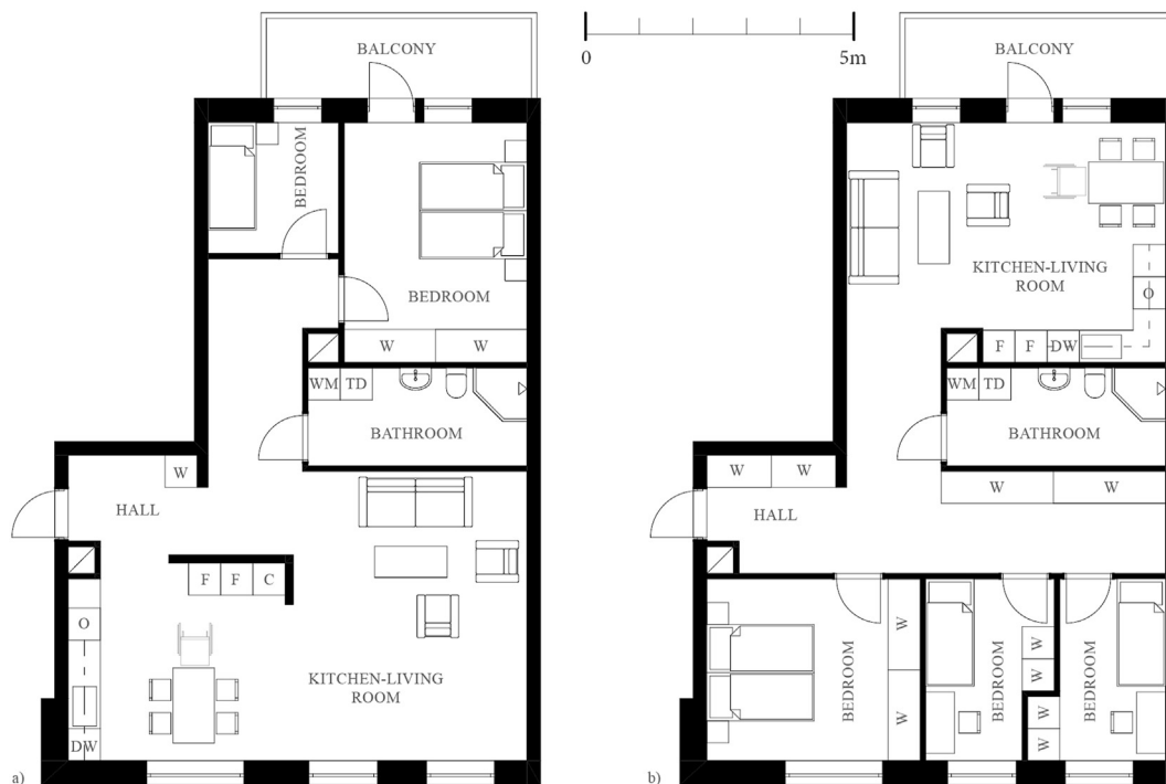
Fig. 12 Exemplifying the concept 'relocate': (a) An apartment floorplan (75.6 m 2 ) with the planned location of the kitchen (Source: illustration by Anita Ollár, original floorplan by Tengbom). (b) A possible relocation of the kitchen (proposal by Anita Ollár). C: cupboard, DW: dishwasher, F: fridge and freezer, O: oven and stove, TD: tumble dryer, W: wardrobe, WM: washing machine.
