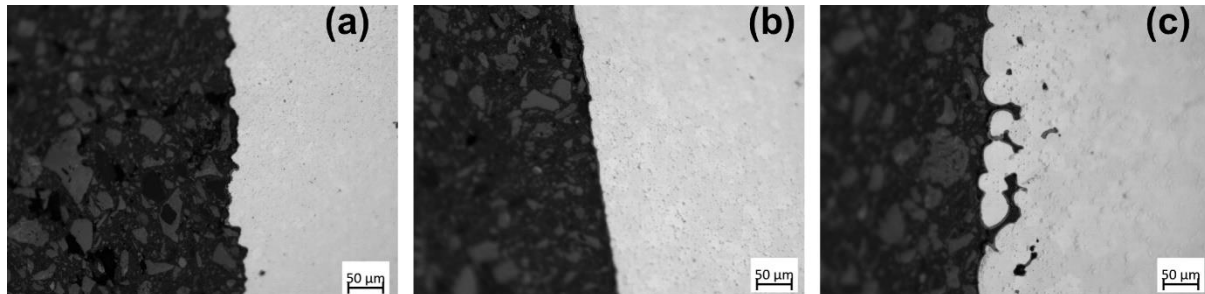
Figure 14 Pore morphology of Vanadis 4E material after sintering at (a) 1150 °C, (b) 1200 °C and (c) 1250 °C and followed by capsule-free HIP
