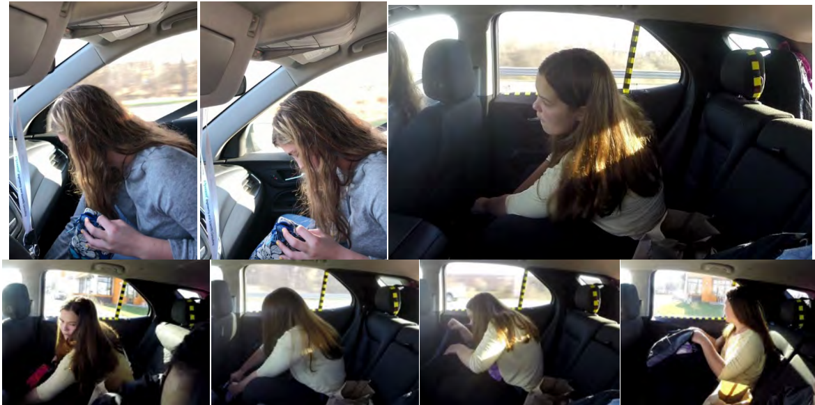
Figure A6: Female volunteer seating positions and postures while grabbing objects from schoolbag in footwell area (activity 3).
