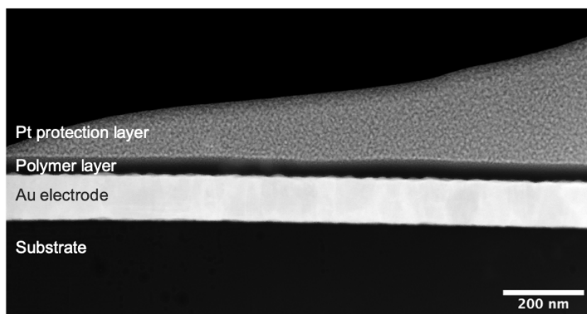
Figure 4.2: ADF-STEM image recorded at 200 kV acceleration voltage showing the different layers of the spin coated bilayer p(g_42T-T):BBL on a Au electrode. A protective layer of Pt was deposited on top of the polymers.
