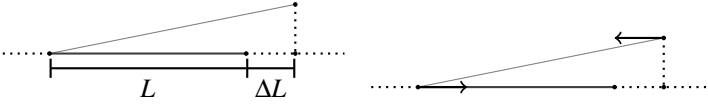
Figure 2.7: The thick lines are the initial edges and the thin lines are their displacements. The left figure shows how the difference in length is calculated by projecting the displaced nodes onto the fibers initial axis and the right shows the forces arising from the displacement.
