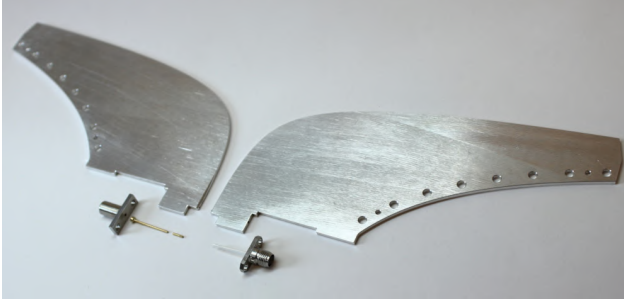
Figure 3.3: Coaxial single-ended excitation feed-through for a ridge-pair.
