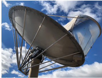
Figure 1.6: Reflector in the Allen Telescope Array (ATA) with shroud shielding against ground. Image credit: Alex Pollak, ATA/SETI.
