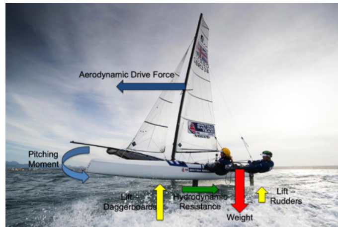
Figure 1. Longitudinal balance of forces on a NACRA 17 foiling catamaran.
