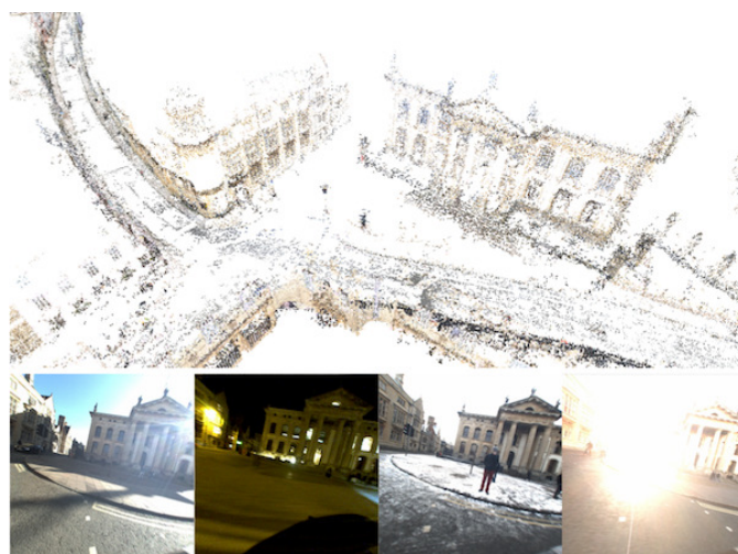
Fig. 1. Visual localization in changing urban conditions. We present three new datasets, Aachen Day-Night , RobotCar Seasons (shown) and Extended CMU Seasons for evaluating 6DOF localization against a prior 3D map (top) using registered query images taken from a wide variety of conditions (bottom), including day-night variation, weather, and seasonal changes over long periods of time.
