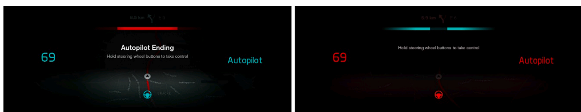
Fig. 2. The HMI view for the TOR (left). The HMI view when the two steering wheel buttons are being pressed; the turquoise bars are moving toward each other (right).
