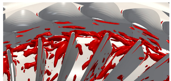
Fig. 16. Complex vortical structures behind guide vane trailing edges at minimum load condition. Iso-surface of \lambda_2 = 7500 \text{ s}^{-2} .
