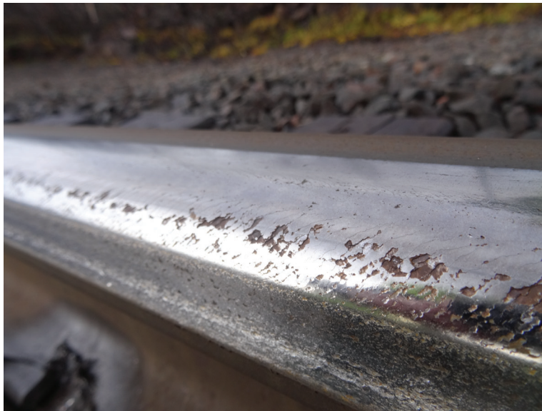
Figure 1.1: Gauge corner RCF cracks of a rail. Photo: Anders Ekberg.
