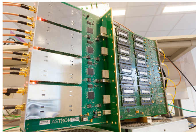
Fig. 21. Analog to digital conversion board (left), midplane (centre), and UniBoard (right), cover removed.
