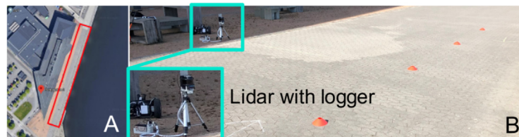
Fig. 4. Experimental setup. Panel A: Birds-eye view of the field trials. Panel B: Setup of the LiDAR and the cones (for the steering trial).
