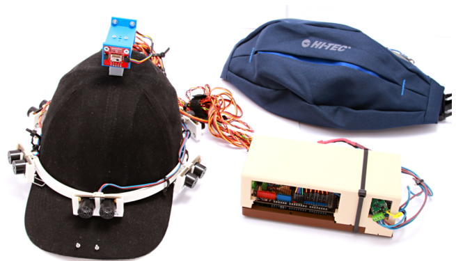
Figure 6: The prototype of Gapeau: the sensing hat (left) is connected to a control unit (bottom right), which is worn in a belt-case (top right) on the user's back.
