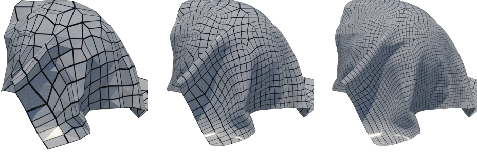
Figure 2.2: An object represented with quads, with an increasing level of tessellation from left to right.
