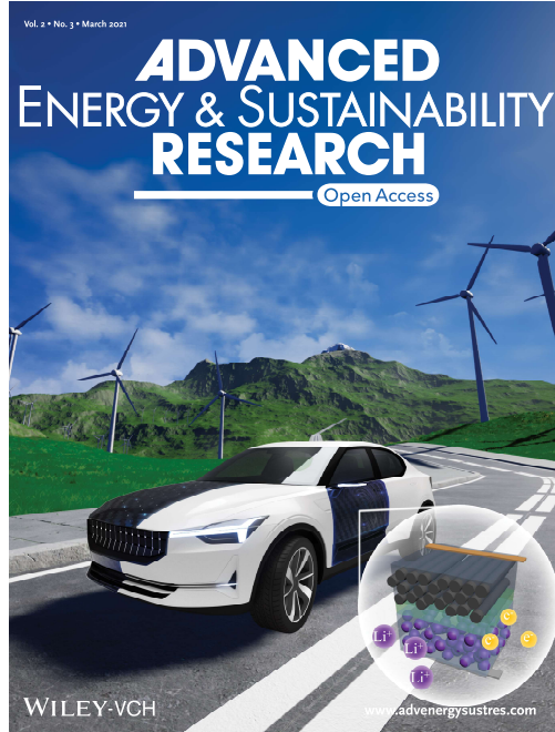
Figure 1.1: The structural battery composite concept: a multifunctional composite material capable of simultaneously carrying mechanical load and storing energy (i.e. work as a battery). This image is a reprint of the back cover page for Paper A , [16].
