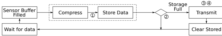
Figure 4.9: Execution flow of a data collection application which benefits from compressed I/O.
