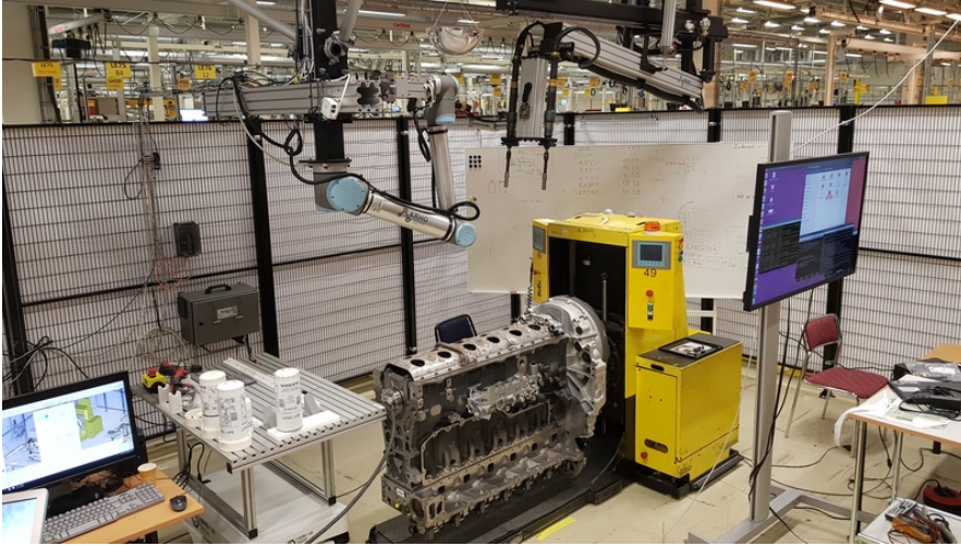
Figure 2: Collaborative robot assembly station controlled by a network of ROS2 nodes. A video clip: https://youtu.be/TK1Mb38xiQ8 .
