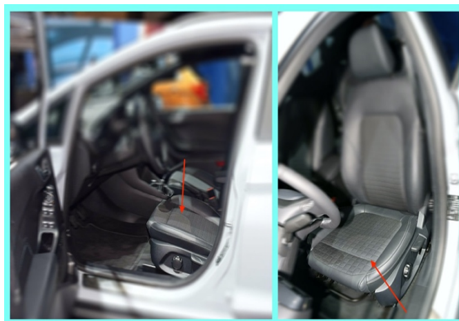
Fig. 3: The view of a car seat cushion presented for the perceived comfort evaluation with the blurred interior parts.
