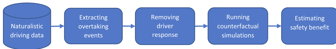
Fig. 1. Methodology overview for safety benefit estimation of FCW for car-to-cyclist crash avoidance in overtaking manoeuvres.
