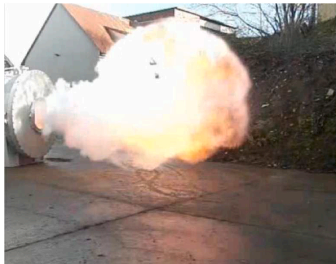
Fig. 2. Vented corn starch dust explosion in the 11.5 m 3 vessel.
